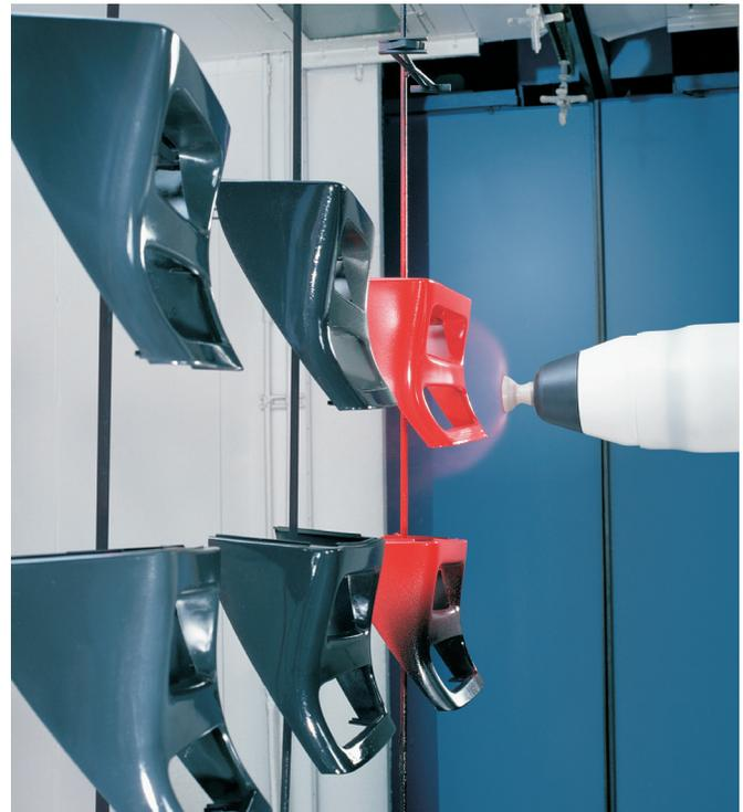
The production-proven Nordson RA-20 rotary atomizer delivers painting efficiency and superior finishing quality and operating safety for a wide range of finishing applications. Unlike conventional painting bells, the patented RA-20 has no minimum sparking distance. As a result, it can be positioned close to parts for optimal coverage and minimal overspray.
