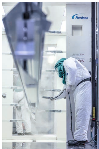
The complex profiles are sprayed before or after the coating process with two hand-held guns in order to ensure the best possible coverage.
