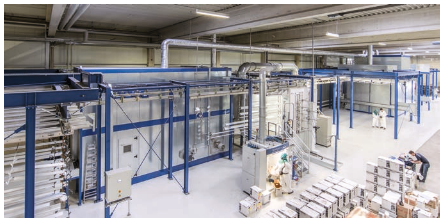
An overview of the new powder coating shop. In the centre of the picture is the pre-treatment line and next to it the fast colour change spray booth with the powder feed centre. On the right is curing oven.
