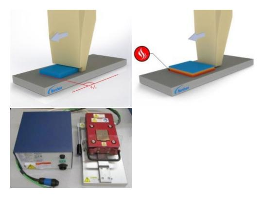
Low profile die shear testing is required when the die under test are very thin and their height profile is low relative to the surface that they are bonded to. A relatively high force die shear load cartridge combined with high precision shear height accuracy and a self-aligning load tool are critical.
