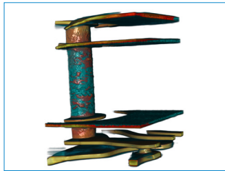
Section of via showing plating variations
