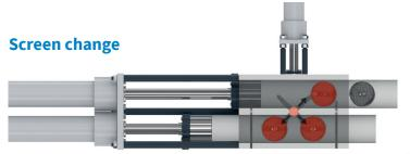
The screen change takes place when the self-cleaning is completed. The screen piston with the filter element to be cleaned is moved out of the housing, far enough to allow for the screen pack to be removed and replaced with a new filter element. During the screen change, three screen cavities (75%) remain in production. The screen change proceeds for all four screens successively.
