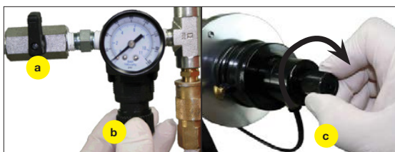
HSS regulator air pressure Fluid pressure adjustment
