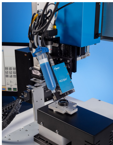
Fixed head creates less wear and tear with the rotating table.
