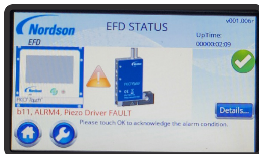
The system displays the alarm code (in this case, b11 004, Piezo Driver Fault).
