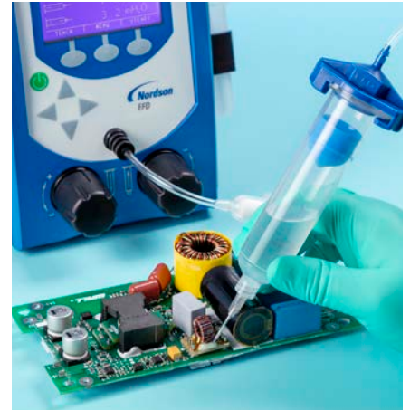
The Ultimus II provides the most control when dispensing watery CAs.
