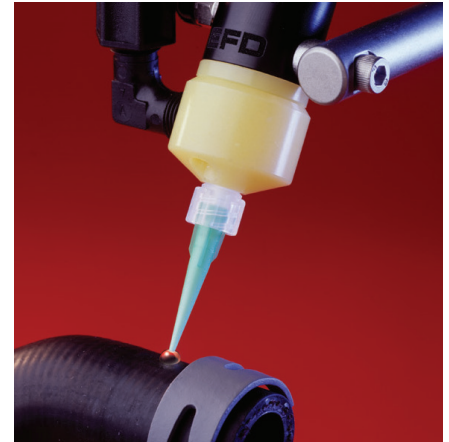
Tip selection is critical to the success of cyanoacrylate applications.
