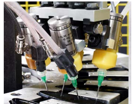
Install dispense valves in-line for high volume production.
