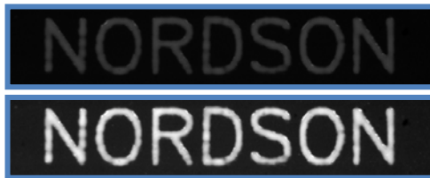
Example of Software Programmable Camera Gain Adjustment
