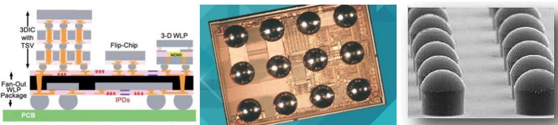
Figure 1 Advanced packaging processes integrate chips and substrates vertically to put more power and functionality in less space. Many advanced packaging processes use solder bumps and pillars for vertical connections. Source: Yole Development, Amkor.
