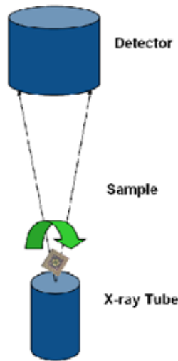
Figure 4. Typical \mu CT set-up used in the electronics industry. The sample is suspended between the X-ray source and detector. 2D images are taken at multiple angles by rotating the sample.
