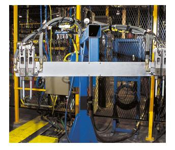
Magnetic proximity switches within the gun sense fullydispensed and fully-loaded conditions. Switch actuation failure signifies a fault condition, indicating that the dispense shuttle did not reach either a filled or dispensed stop. In this case, an alarm can be activated to warn of a faulty dispense shot or gun malfunction.
