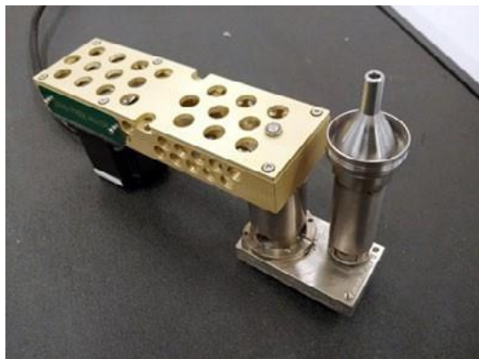
ControlFlow system with grooved riser and sleeve
