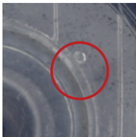
Lens Inspection - Bubble Defect
