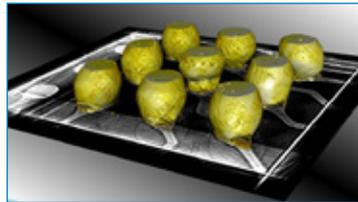
3D visualization using X-ray CT shows head in pillow defect and solder ball cracking
