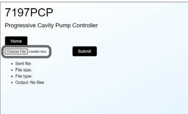
Update screen after the firmware update file is loaded (the firmware update file name is shown next to the Choose File button)
