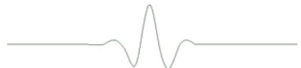
Ultrasonic signal from a thin wall tube
