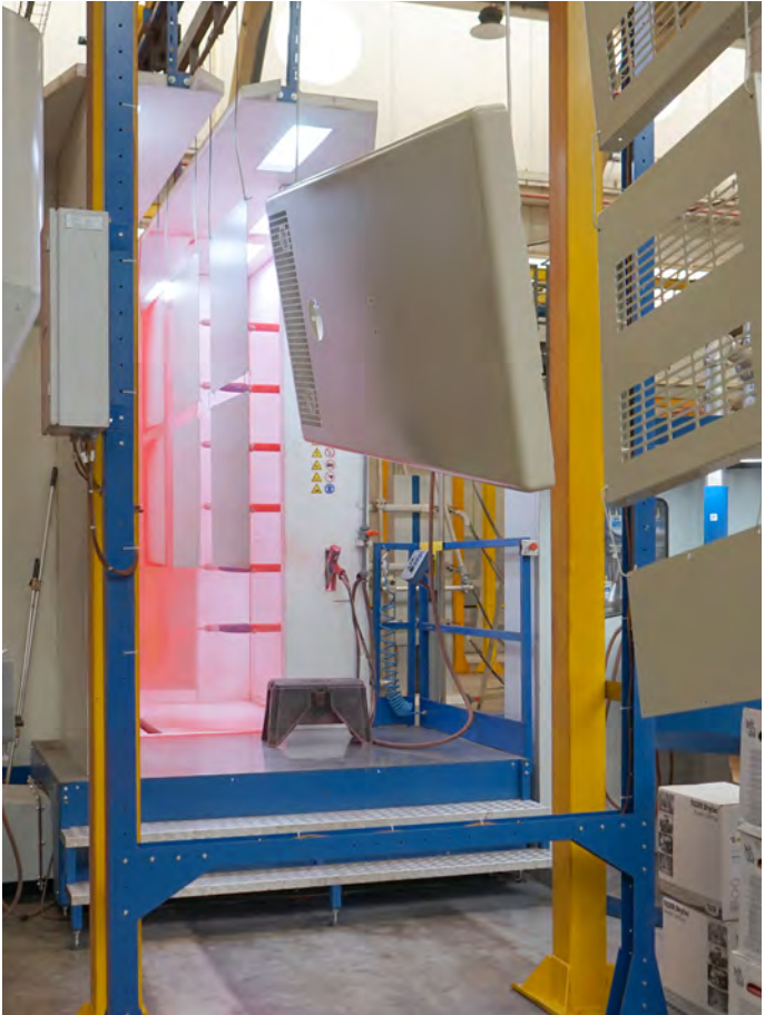
With the new powder coating system, a coating thickness of 60 µm as well as 120 µm is achieved, depending on the product and use.
