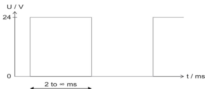
Oscilloscope (valve output) for a Liquidyn P-Jet valve
