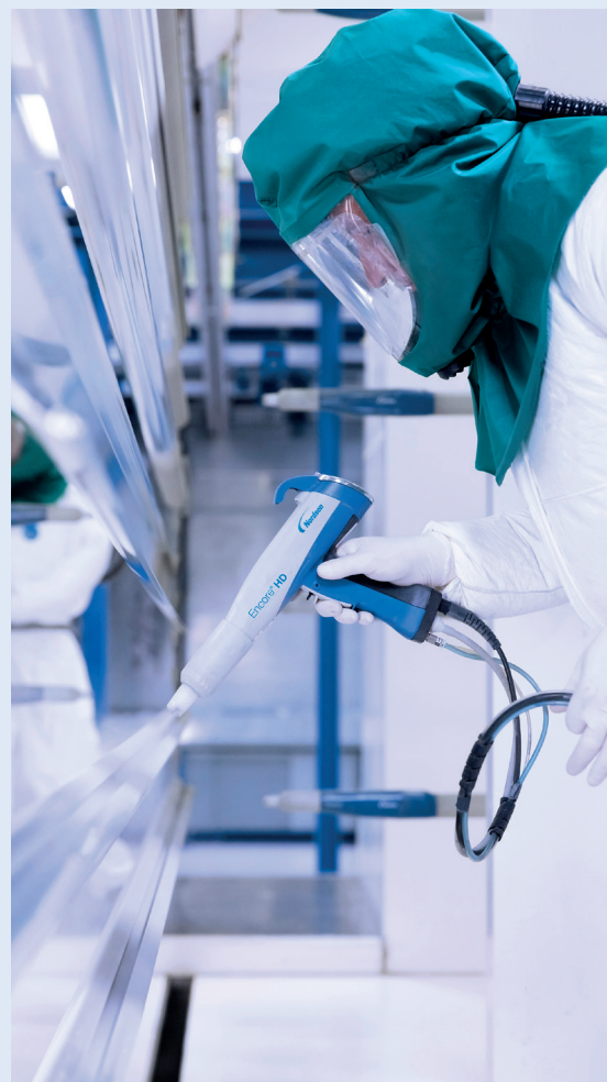
The soft spray at low velocity improves application efficiency in the initial coating operation.
