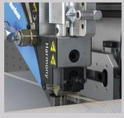
Nordson Allegro™ nozzles efficiently apply adhesive to single or multiple elastic strands using novel air-assisted contact coating technology to wrap adhesive completely around the strands. Allegro nozzles provide: Optimal adhesive placement
