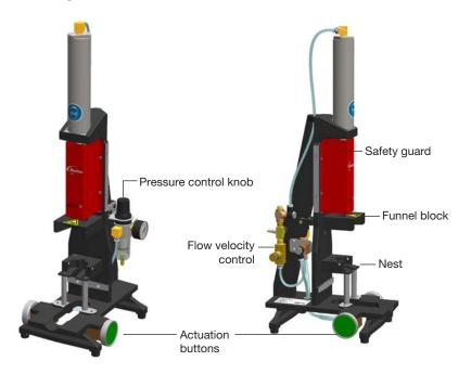
The Atlas 2K Piston Inserter was specifically designed for ONE operator to insert EFD AF Air Free pistons into EFD 2-component (2K) cartridges. During operation, a filled cartridge is placed in a nest underneath a block loaded with two pistons. Simultaneously pressing the two actuators causes a pneumatic cylinder to descend and press the pistons onto the cartridge.
