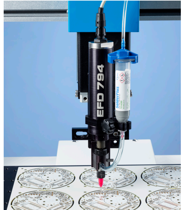
794 auger valve and robot dispensing solder onto a fire detector.
