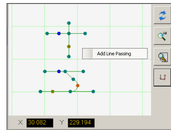
Right-click to stitch a Line Passing point onto an existing point
