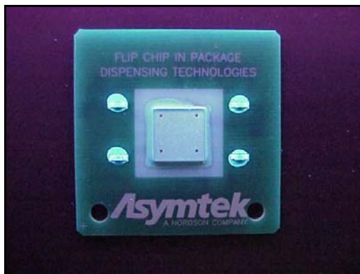
Jet-Coated 0805 Resistors Around Underfilled Chip
