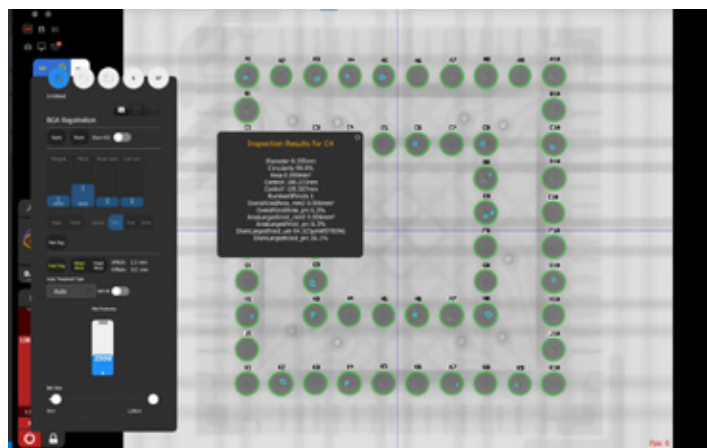
Figure 5: Detailed inspection results of individual BGA ball.
