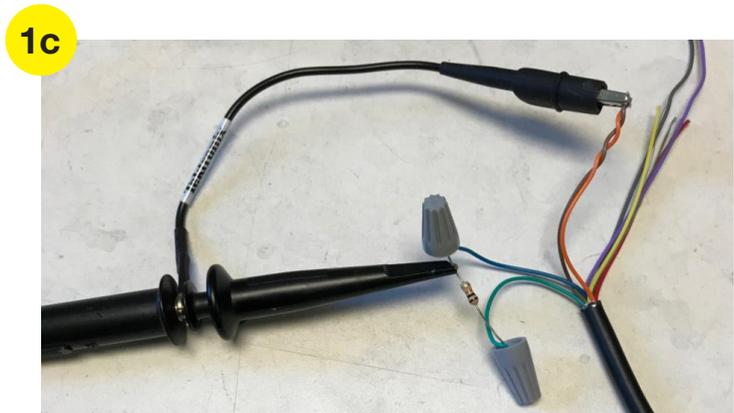
Oscilloscope connection example
