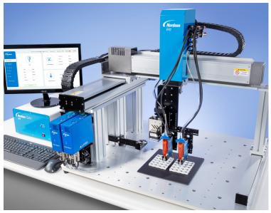
Engineering enhancements to the GVPlus solution enable the product to provide positioning accuracy and deposit placement repeatability at  $\pm~0.008$  mm / 8  $\mu m$ .
