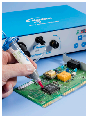
Dispensing SolderPlus® solder paste on PCB boards.
