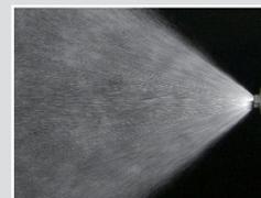
*Pattern collapse with PermaFlo® 830 pump*
