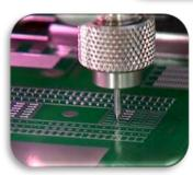
The DV-8000C Heli-Flow Pump with fixed-head design excels at dispensing high-viscosity fluids and high flow rate for higher speed dispensing.
