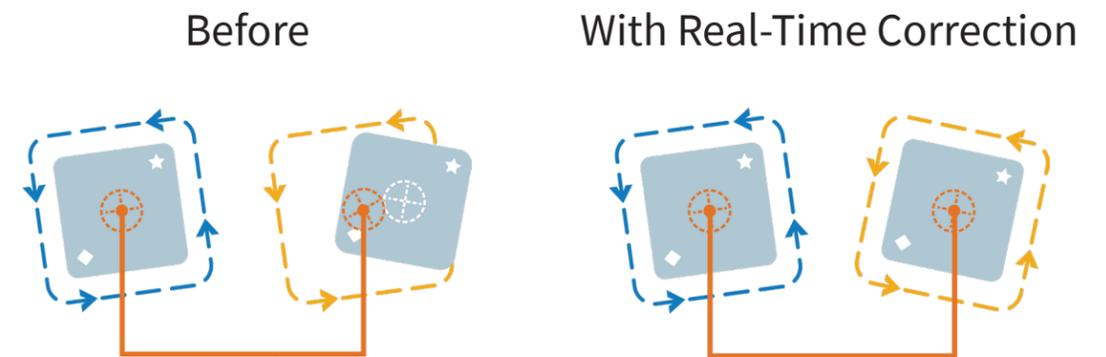
Early fixed-pitch, dual-valve designs could not adjust for individual part-to-part skew, negatively impacting yield.
