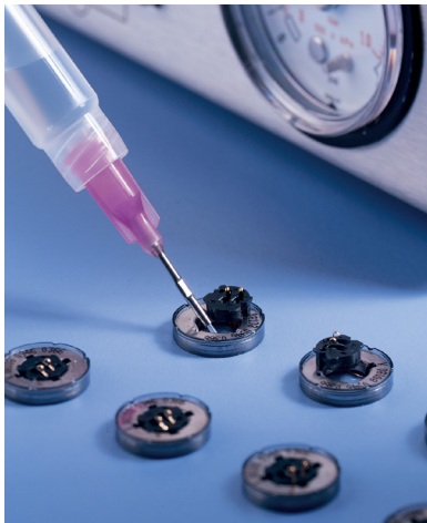
Precise cyanoacrylate deposits with EFD systems
