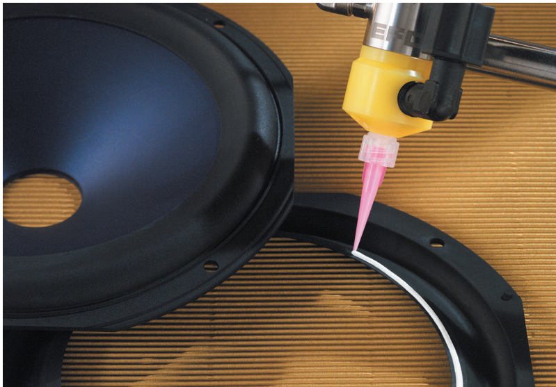
752 diaphragm valve dispensing adhesive bead on loudspeaker components.
