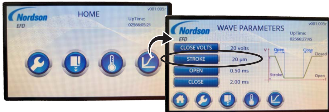
WAVE PARAMETERS screen on the Touch XP controller (STROKE units set in microns)
