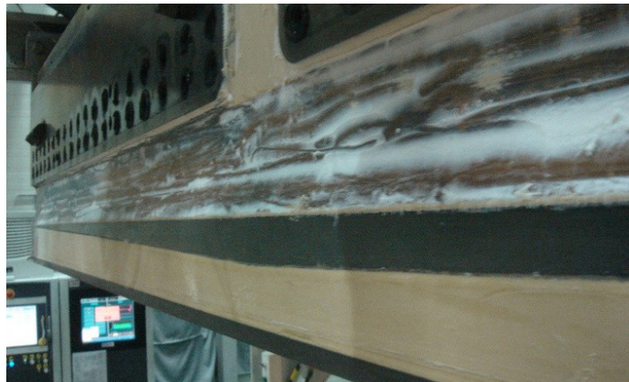
Figure 3: Residual degraded material adhered to the flow channel, requiring frequent cleaning to avoid defects.
