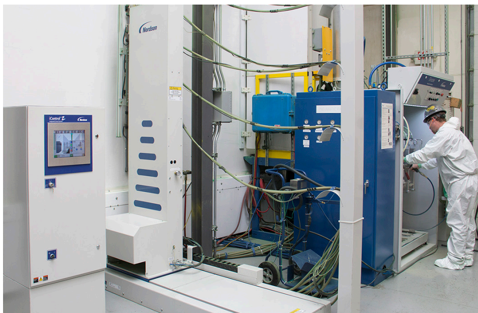
An operator performs a color change from light to dark powder in the second ColorMax® system.
