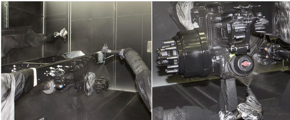
Trilogi® automatic electrostatic spray gun applies two-component coating in spray booth three.
