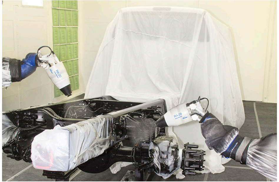
Robot rotary atomizers apply rust-inhibiting, two-component coating to the vehicle framework in spray booth two.
