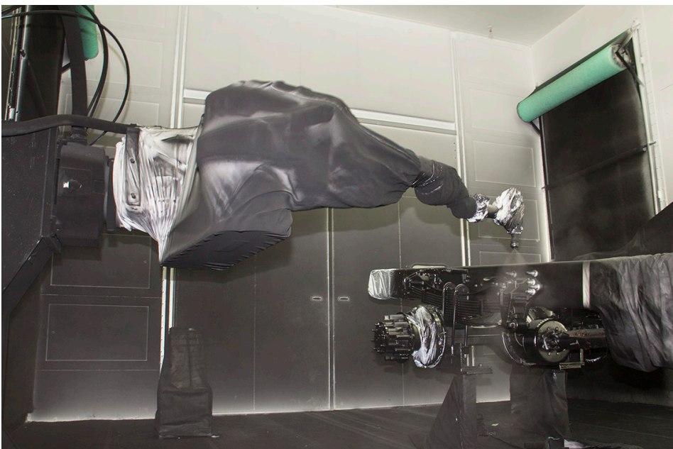
Trilogy® automatic electrostatic spray gun applies two-component coating in spray booth three.
