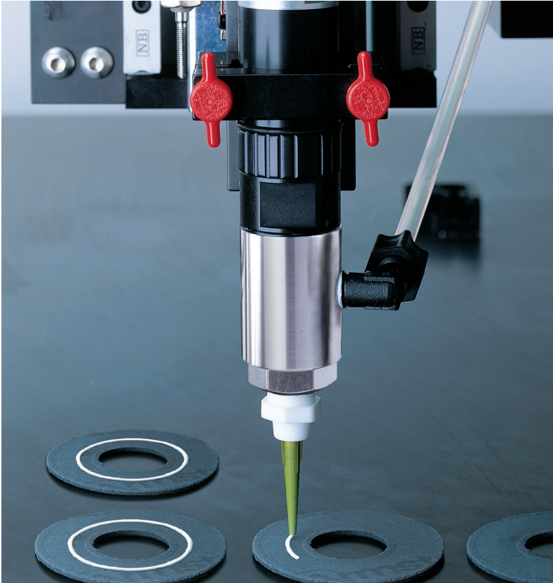
725DA dispensing even bead of water-based adhesive.
