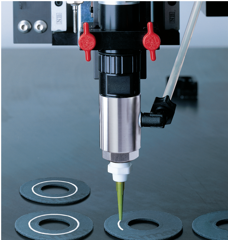
725DA dispensing even bead of water-based adhesive.
