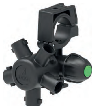
3-4-5 way nozzle holder with diaphragm check valve • Specific for high flow rates Stainless steel screw and nut are included
