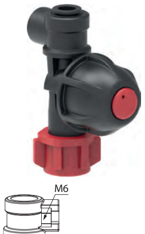
Nozzle holder with quick coupling for hose Ø 8 mm, check valve and threaded cap 3/8"
