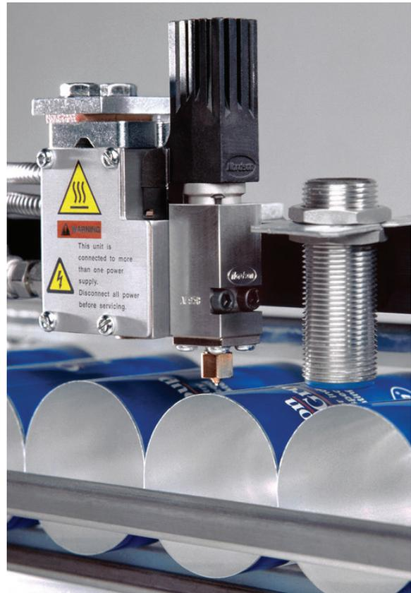
Controlled application also promotes clean tooling by preventing excess lubricant from building on equipment. The cleaner environment extends periods of operation between line clean-ups and minimizes line stoppages caused by excess lubrication.
