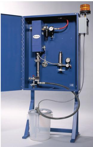
A five-gallon container, interfaced with the fluid level controls, holds the lubricant. The system's pump also provides dual-acting reciprocation for consistent material flow and minimized pressure winks. In addition, a low-pressure regulator maintains the spray pressure supplied to the gun from 0 to 80 psi, resulting in more uniform bead deposition.
