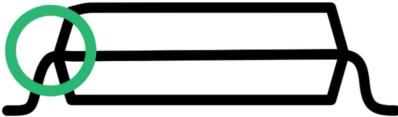
**Figure 1:** Side profile of SOIC20 microcontroller with knee highlighted in green
