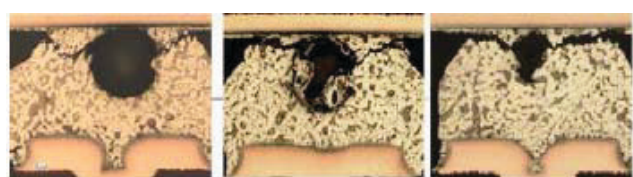
ENIG 1x Reflow – Examples of void-assisted solder fatigue cracking
