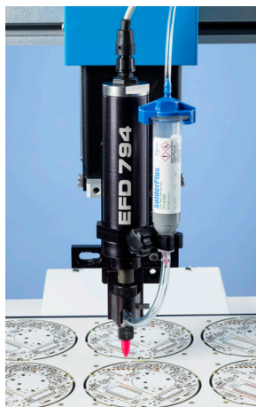
794 auger valve dispensing EFD SolderPlus paste onto a fire detector.
