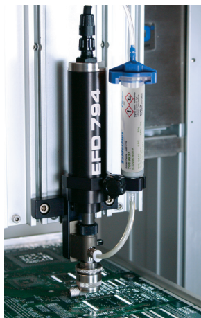
794 auger valve dispensing EFD SolderPlus paste onto a printed circuit board.
