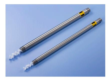
Series 85 Pipe Mixers are designed for high-pressure applications and feature sturdy metal housings with Series 120 disposable plastic mixing elements. The housing is made from heavy-walled stainless steel pipe that resists dents and distortions. For routine maintenance, the mixer can be pushed out and replaced.
