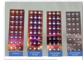
Figure 6 Appearance of Bare Copper lead frame after plasma treatment
