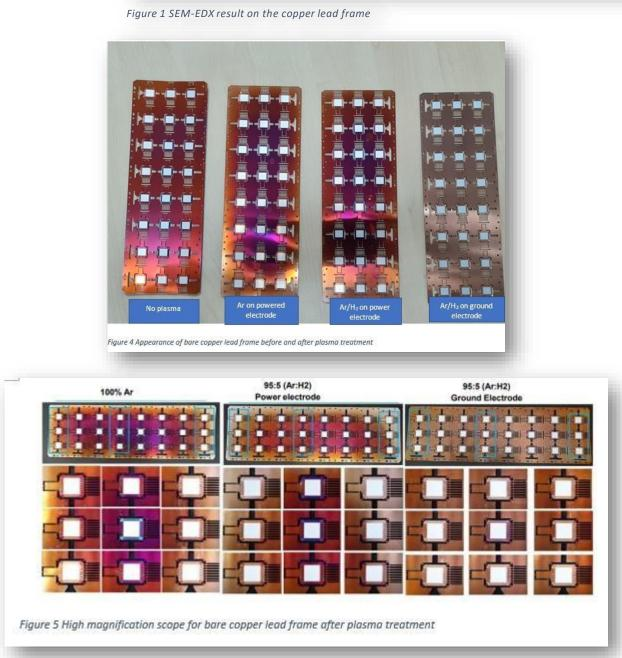
The pre-plasma treated lead frame was observed to be discolored after the heat exposure in the different process steps. Discoloration was still found on samples treated with Ar on powered electrode and with Ar/H<sub>2</sub> on a powered electrode setup. However, there was no discoloration observed on the lead frame after treatment with Ar/H<sub>2</sub> on the ground electrode setup
