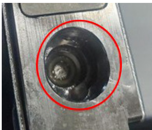
Examples of Pulse valve actuators with UV adhesive contamination in the push-rod cavity
