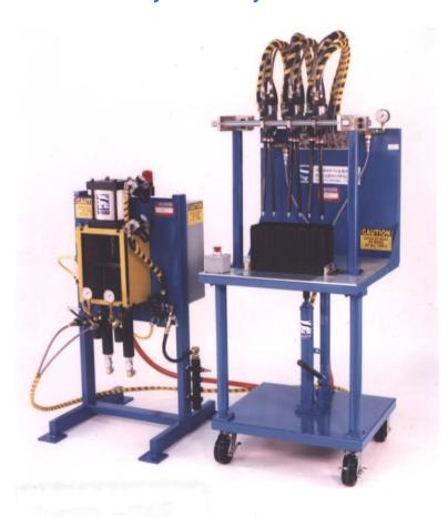
Battery manufacturers bond battery elements into each cell. This automated battery cell application required a preset 'shot' of mixed epoxy - in rapid succession, into each of 6 battery cells.
