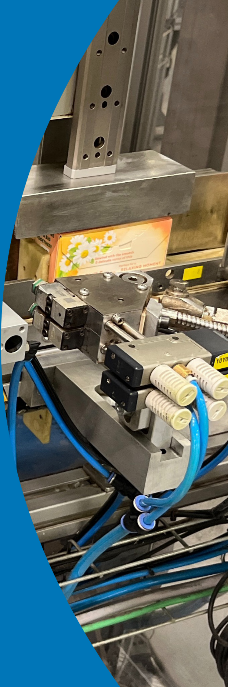
Ensuring the precise sealing of the top cardboard flap with adhesive is crucial.
